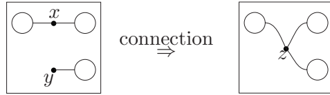
Figure 4: The connection operator in Yoshida’s process graphs partitions the named nodes and immediately renames them. In the graph illustrated, x and y have been related and renamed z . Instead of trying to do all this in a single connection operator, it is more convenient merely to fuse the names. Renaming can then be left to the standard naming equations shown in Figure 3.
